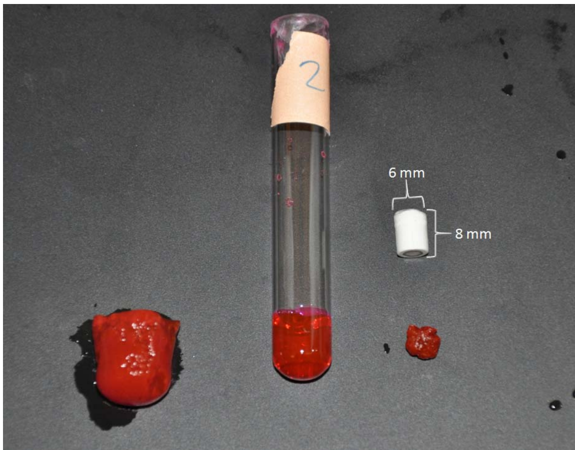
Figure 1-2: Hydrogel in three stages: fully swollen (left), after polymerization with ambient moisture content (center), fully collapsed (right). *Eraser added for size reference*
