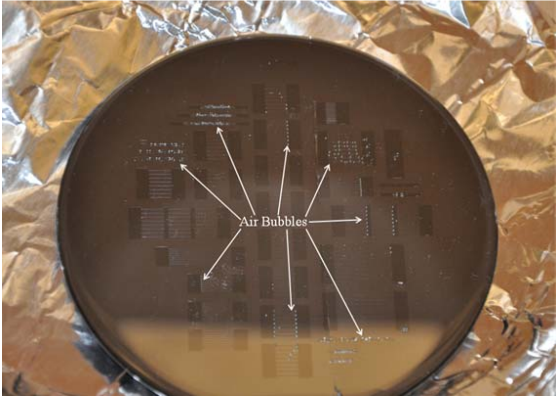
Figure 2-6: Air bubbles in a PDMS stamp still on an SU-8 master mold.
